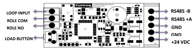
LOOP INPUT: Loop Detector 5-24VDC Live Signal Head
