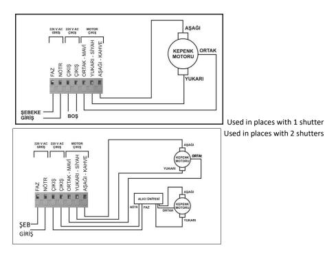
It is used in places with 2 shutters. Button 1 of the controller is loaded to UPS, button 2 is loaded to the receiver unit.
